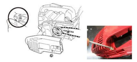
7) Adjust the chain tension by turning the tension screw until the straps touch just the bottom side of the bar.
