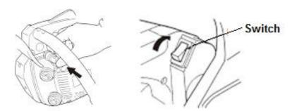
b. Pull the starter button. The starter will close and the throttle will be moved to the starting position
