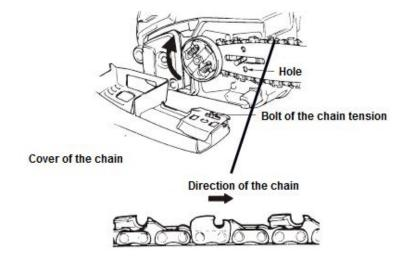
6) Adjust the chain tensioning nut in the lower hole of the guide. Then install the chain and secure the mounting nut.
